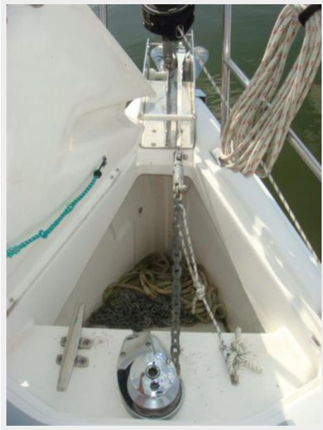
38' Hunter anchor windlass exposed
