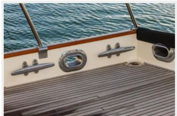
Stainless steel house and cleats
