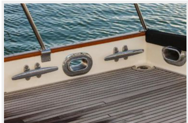
Stainless steel house and cleats
