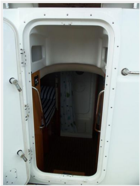
Engine Room Watertight Door
