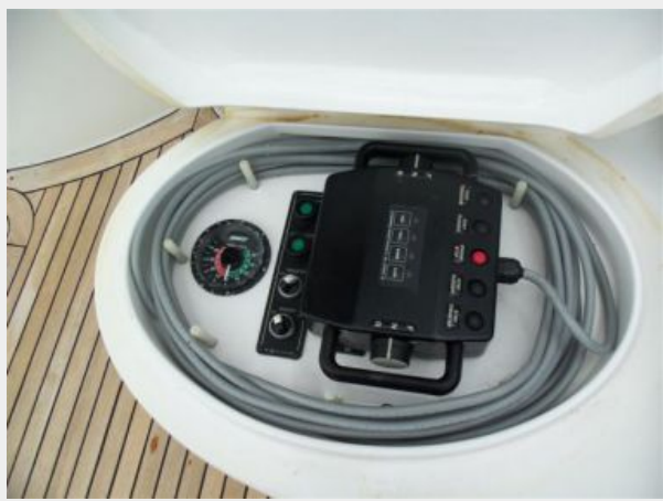
Starboard Side Cockpit Remote Control
