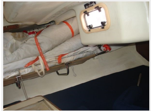
Pipe berths starboard & Port
