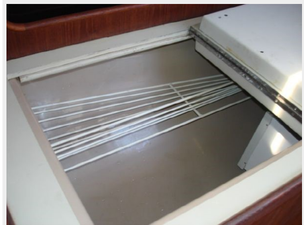
Refrigerated Icebox & freezer
