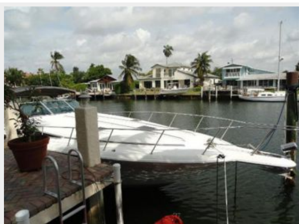
Bow Railing/ Pulpit
