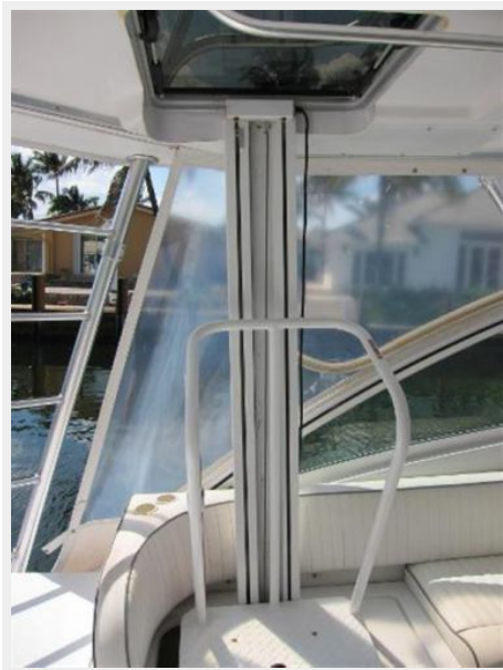
Lift to flybridge
