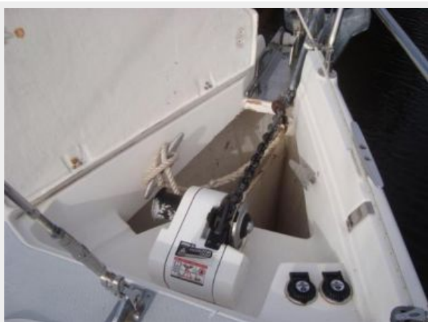
Anchor Locker - Windlass
