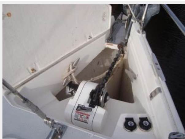
Anchor Locker - Windlass
