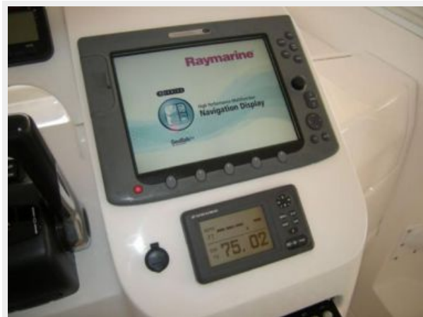
Console Raymarine E120 display, Furuno digital depth display
