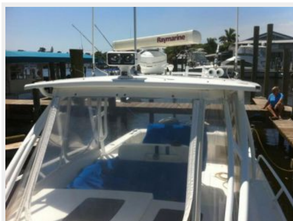
Hard top, radar, antennas, ACR remote control search light
