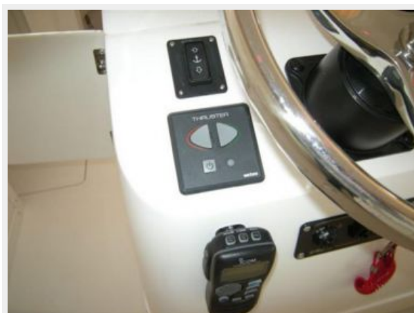
Console, Bow thruster, windlass control, VHF
