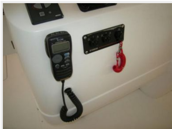
Console, VHF, ignition and kill switches
