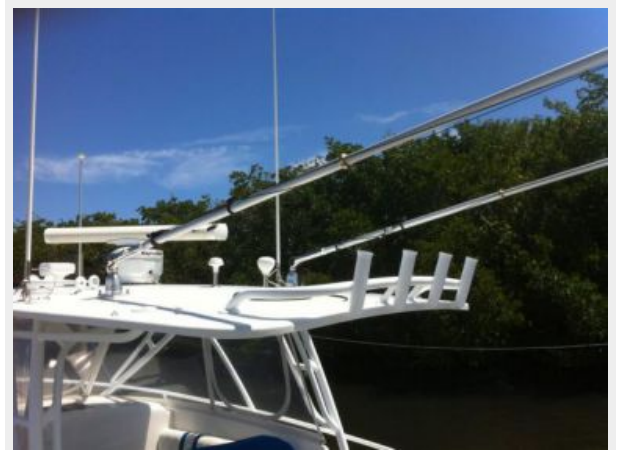
Hard top, radar, outriggers, rod holders, antennas
