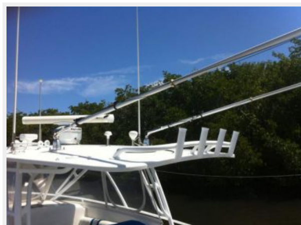
Hard top, radar, outriggers, rod holders, antennas
