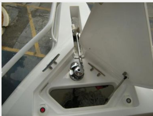
Windlass and anchor rode locker
