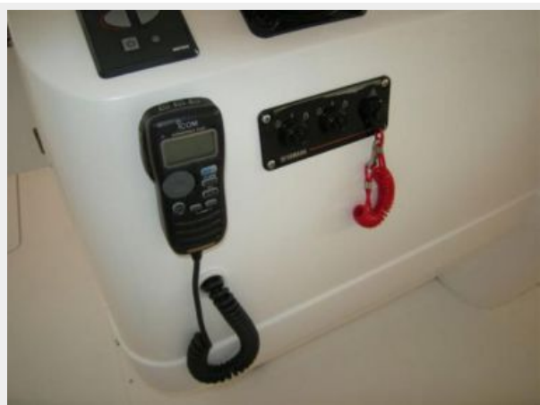
Console, VHF, ignition and kill switches
