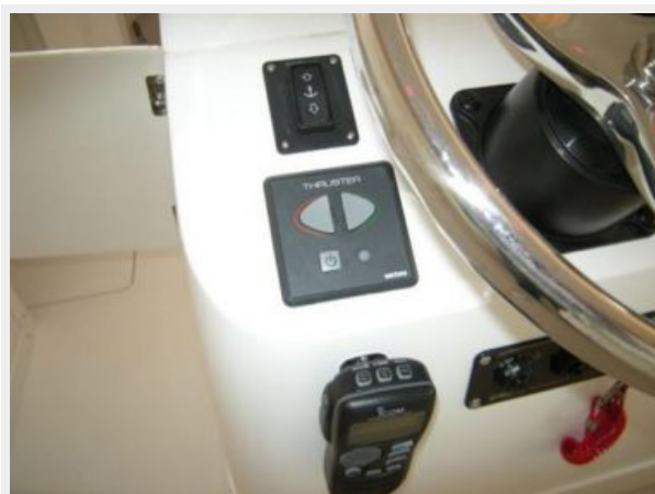
Console, Bow thruster, windlass control, VHF
