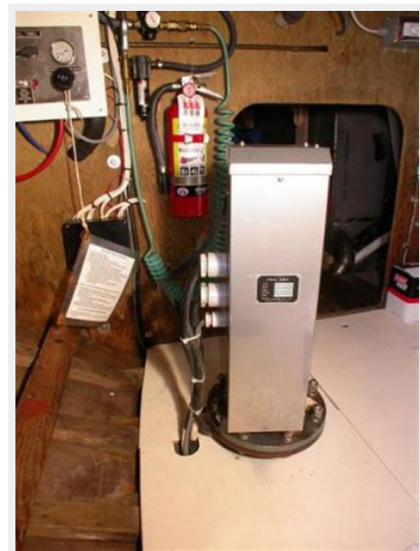
Furuno retractable SONAR
