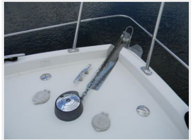
Windlass and Anchor
