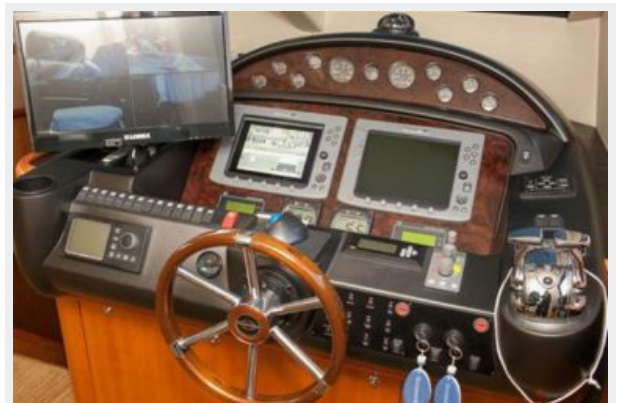
Main Deck Helm Console
