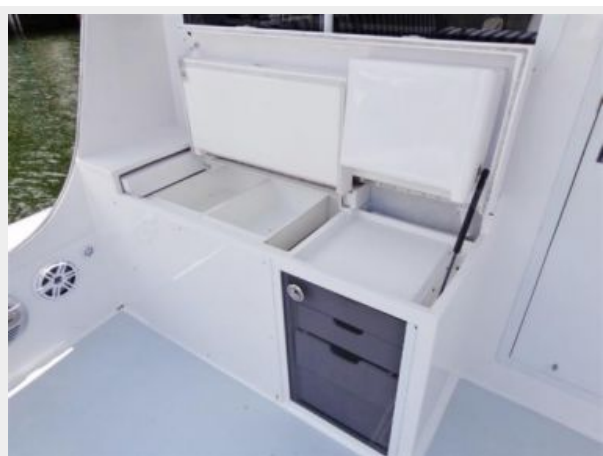
Freezer & Prep Station
