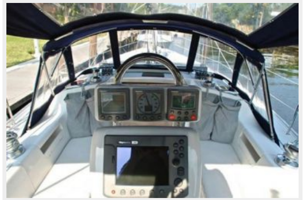
Pedestal Mounted Electronics
