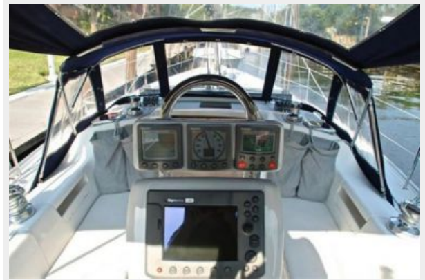
Pedestal Mounted Electronics
