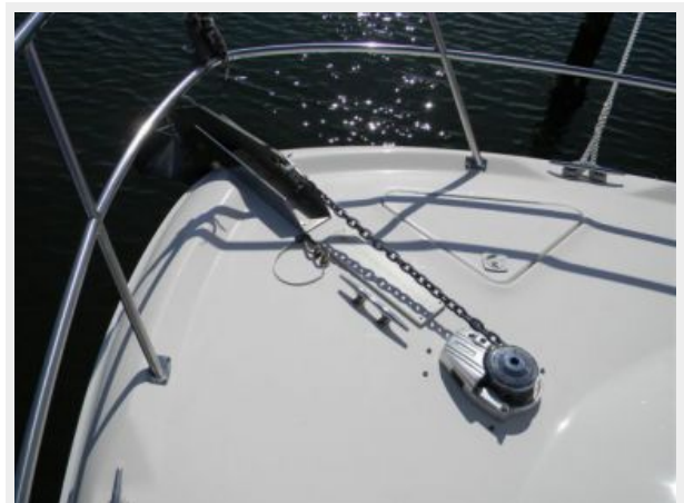
Windlass and anchor
