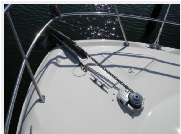
Windlass and anchor
