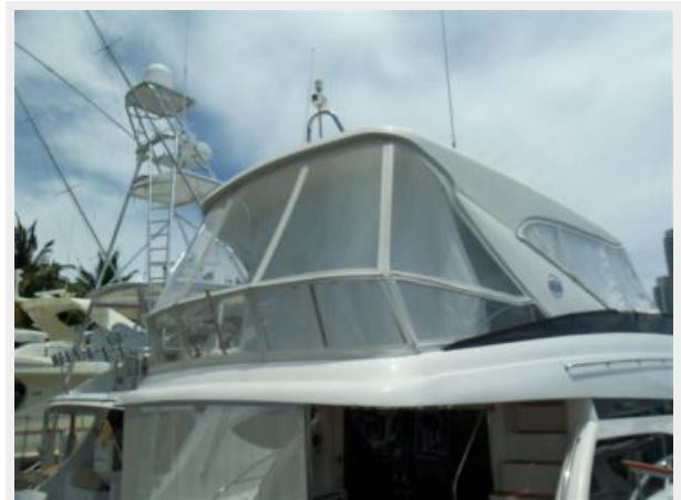
Custom Aft Flybridge Enclosure
