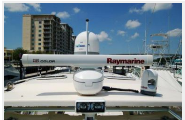
Electronics, Radar, SAT TV and FLIR camera
