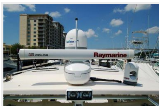
Electronics, Radar, SAT TV and FLIR camera
