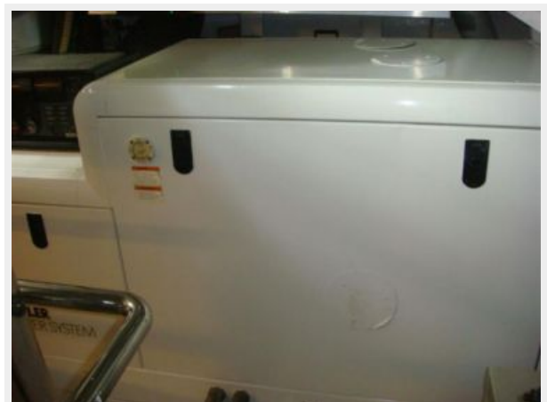
97' Santa Margherita starboard generator sound box
