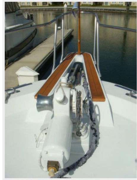
64' Hatteras anchor windlass
