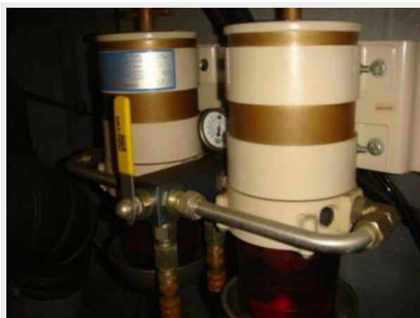
45' Sea Ray starboard Racor fuel filters
