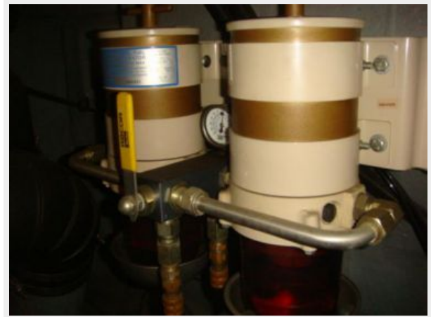
45' Sea Ray starboard Racor fuel filters
