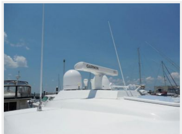
Hard top electronics and antenna
