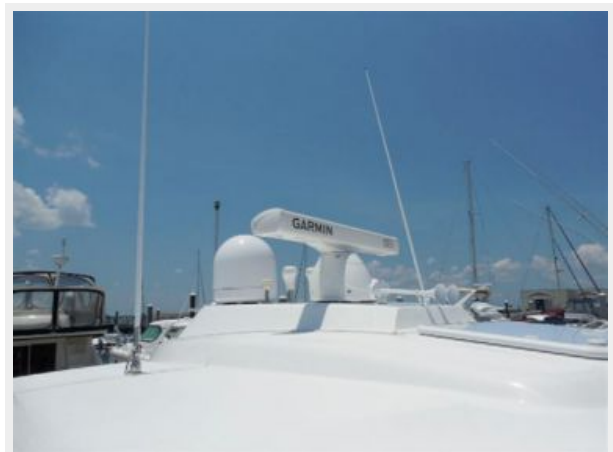
Hard top electronics and antenna
