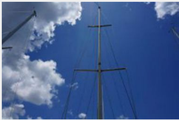
DOUBLE SPREADER RIG
