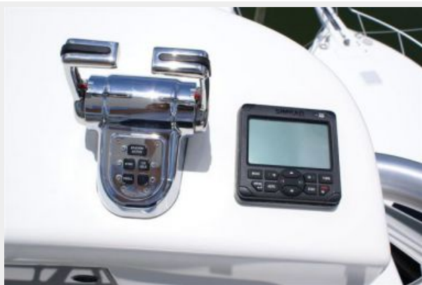
Tower Controls & Autopilot
