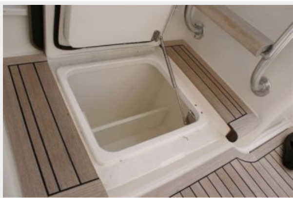
Mezzanine Drink Box/Refrigerator
