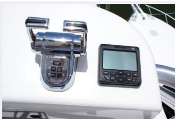
Tower Controls & Autopilot
