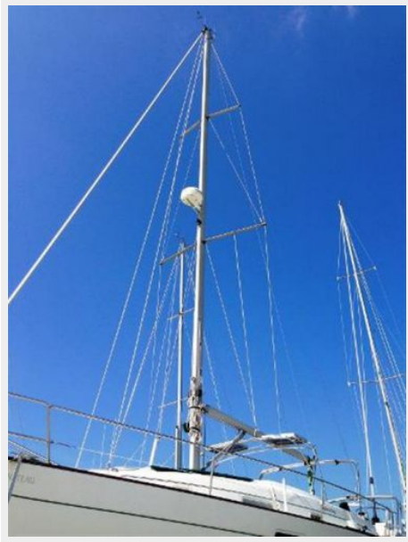
Double spreader rig with radar dome
