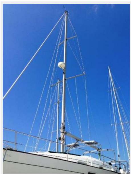
Double spreader rig with radar dome
