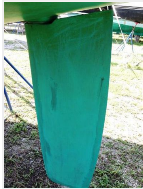
Large rudder with protected bearing
