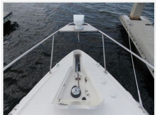
Windlass and Spotlight
