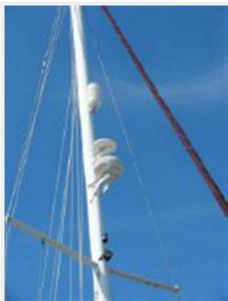
Mast, Radar, Satellite Weather
