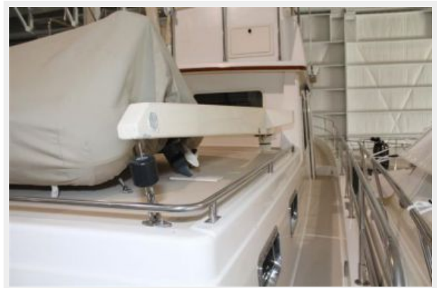
Side Decks & Davit
