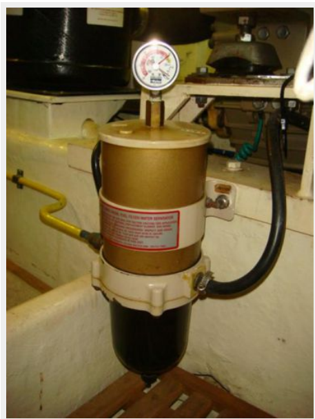
49' DeFever port Racor fuel filter
