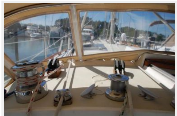
Lines are led aft
