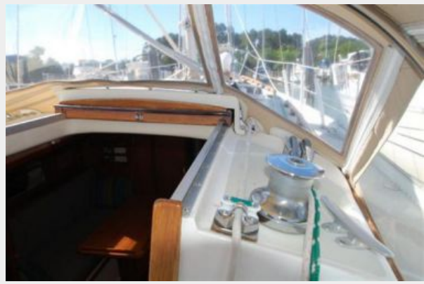
Lines are led aft
