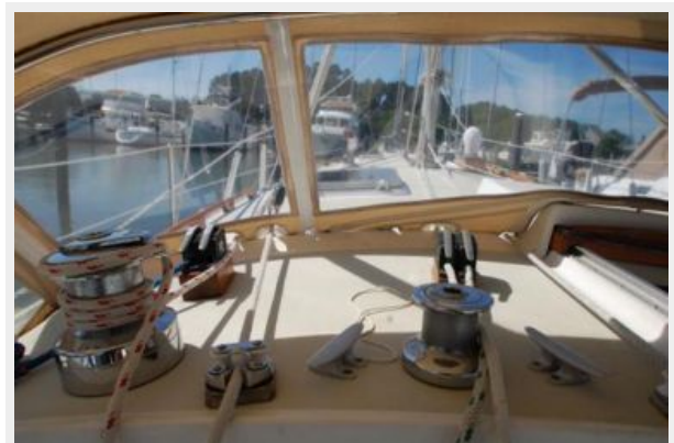
Lines are led aft
