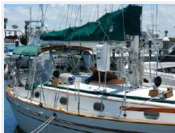
Boom Cradle, Safety Bars at Mast
