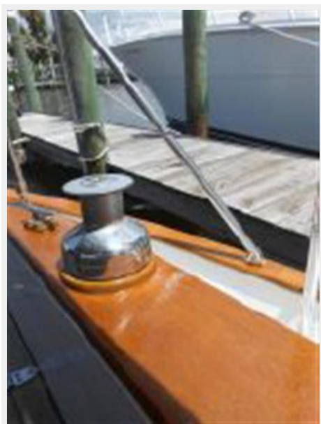
Varnished Coamings and Cap Rails
