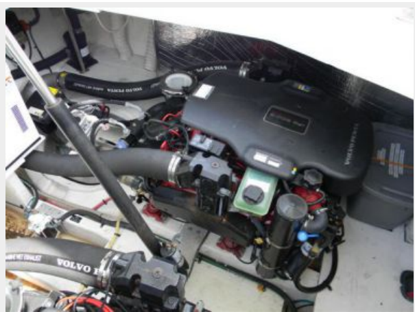
Port Engine and IPS Drive
