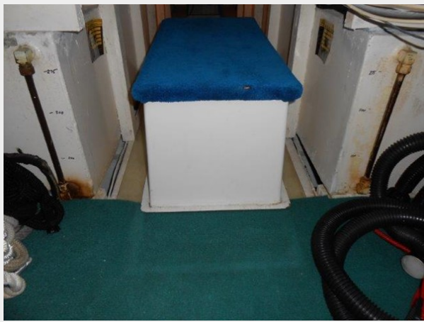
Lazarette Fuel Tanks
