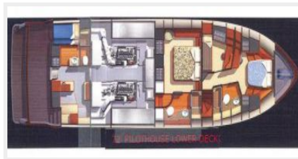
Lower Deck Arrangement
