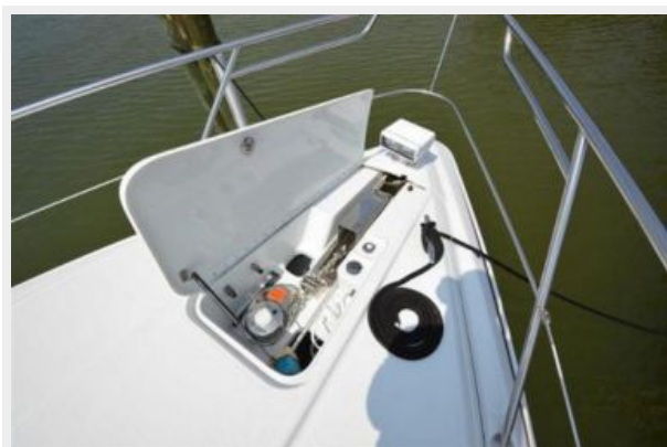
Recessed Windlass Compartment
