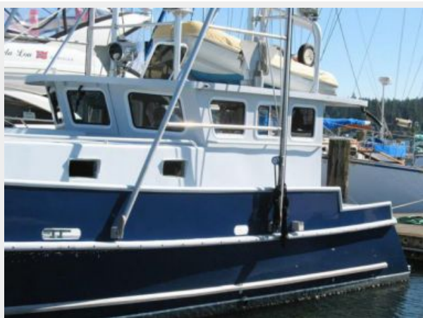
Port outrigger for flopper stoppers
