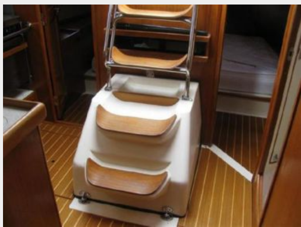
Engine access under companionway steps.
