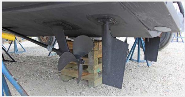
Port Running Gear
