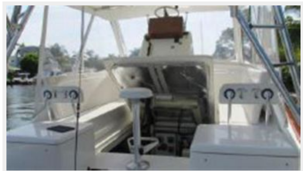
Engine Access Hatch
