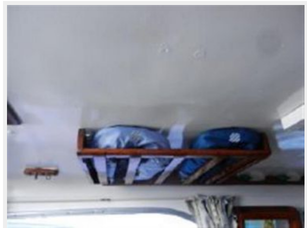
Suspended PFDs in Overhead Rack
