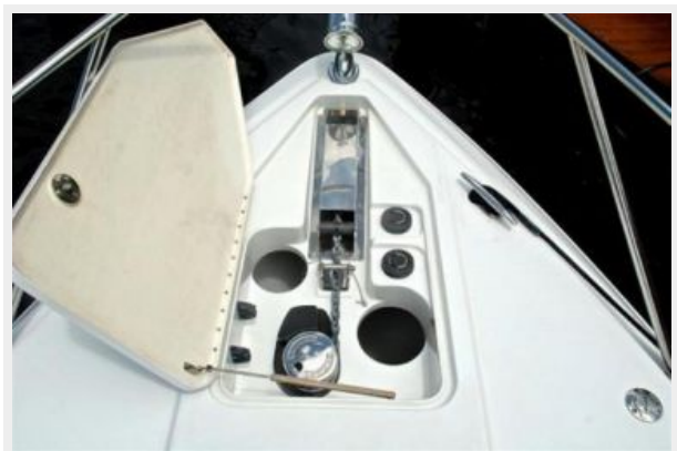
Windlass Anchor Locker
